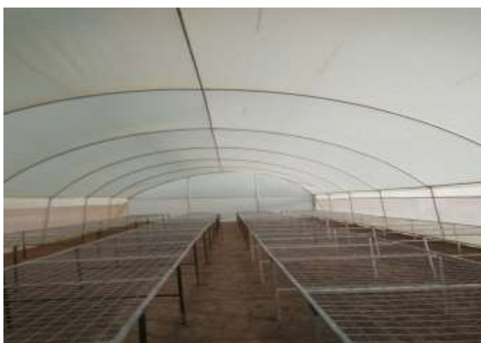
Figure 1.1: Interior of a steel-framed greenhouse with raised seedling beds
