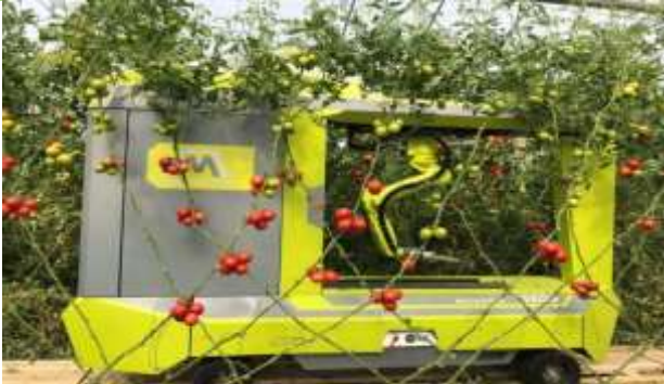
Figure 2.11: MetoMotion's Greenhouse Robotic Worker (GRoW) Harvesting Tomatoes in a Greenhouse. Source: https://www.trendlines.com/company/metomotion/
