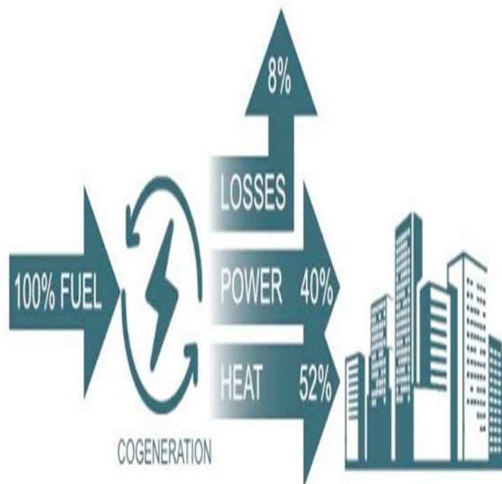
Figure 1: Co-generation energy efficiency Source: Inoplex
